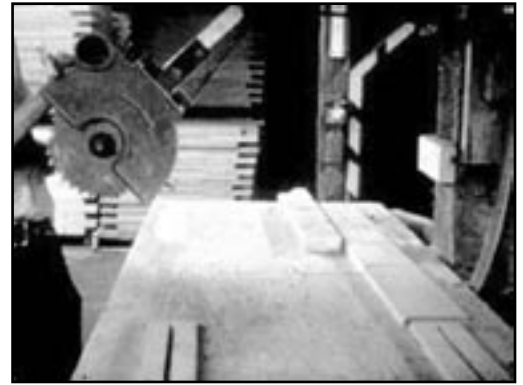
Overhead swing saw missing a lower blade guard and extending beyond table edge.
