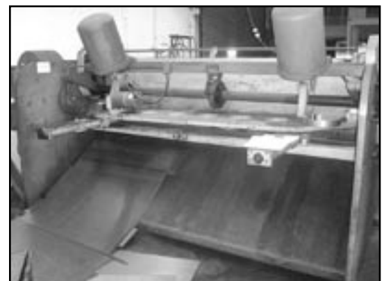
Barricade or restrict the area behind the shear.
