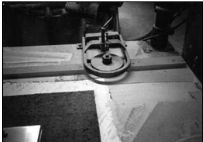
Fence and barrier-type guarding used for straight-line shaping.
