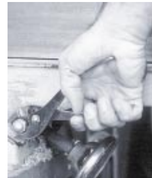
Tool handles digging into the palm and fingers
