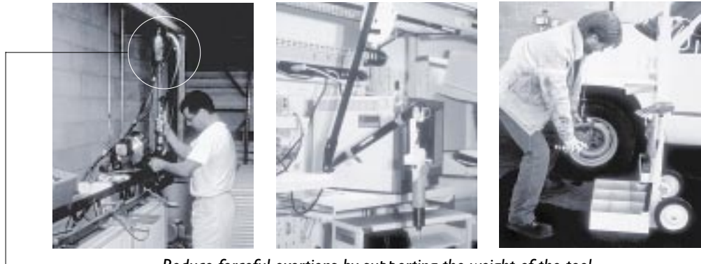
Reduce forceful exertions by supporting the weight of the tool
