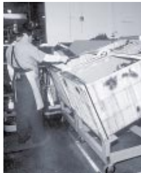
Tilted container with step for easier access
