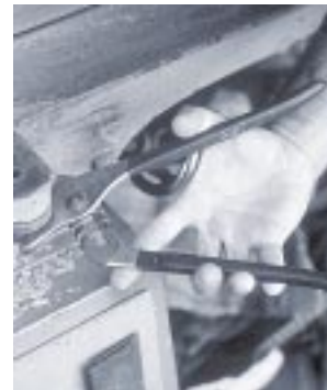
Using a hand tool—grip span too wide
