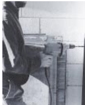
Pistol-grip tool—can be used with a straight wrist on vertical surfaces
