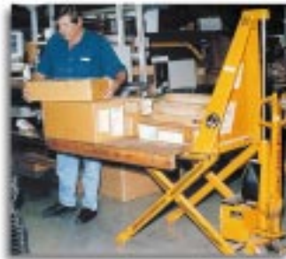
▲ Scissors lift provides a portable, height-adjustable workstation
