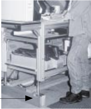
Raise the work surface
